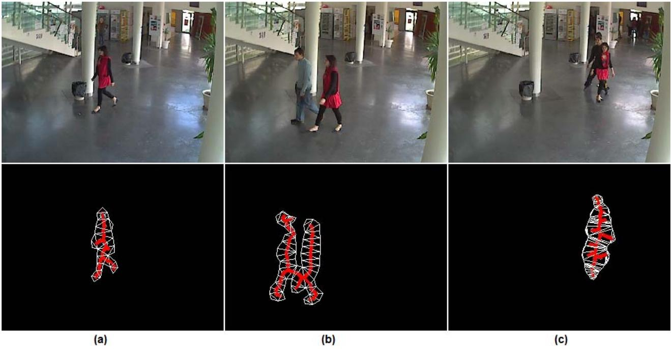
Figure 5. States assigned to blobs: (a) Independent human, (b) Partial Occlusion, (c) Complete Occlusion.
