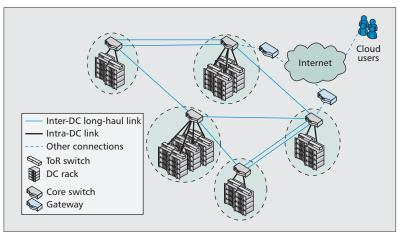
Figure 1. Example of a geo-distributed DC composed of interconnected DC sites.
