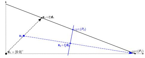
Iteration 2 : an inner feasible solution (contact point)  $\mathbf{x}_2 + t_2^* \mathbf{d}_2$ and a new outer solution. We take  $\mathbf{d}_2 = \text{opt}(P_1) - \mathbf{x}_2$ .
