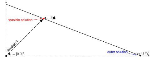
Iteration 1 : found a first outer solution  $opt(P_1)$  and a first inner solution (contact point)  $\mathbf{x}_1 + t_1^* \mathbf{d}_1$
