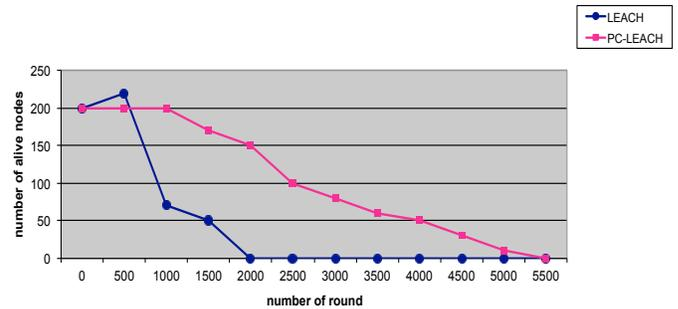
**Fig. 5.** Simulation rounds vs lifetime (300 nodes)
