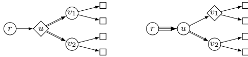
Fig. 1 Two examples of multicast trees with one diffusing node and seven non diffusing nodes. On the left side, u is the diffusing node, and r sends the data once to u , which then copies it twice to v_1 and v_2 , so that those nodes can transmit it to the terminals. On the right side, v_1 is the diffusing node, and r has to send the data three times to u , as v_1 needs to receive the data once and v_2 needs to receive it twice.
