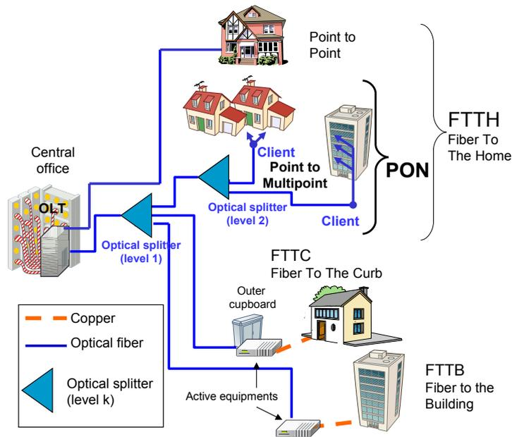
Figure 1: The different FTTx architectures
