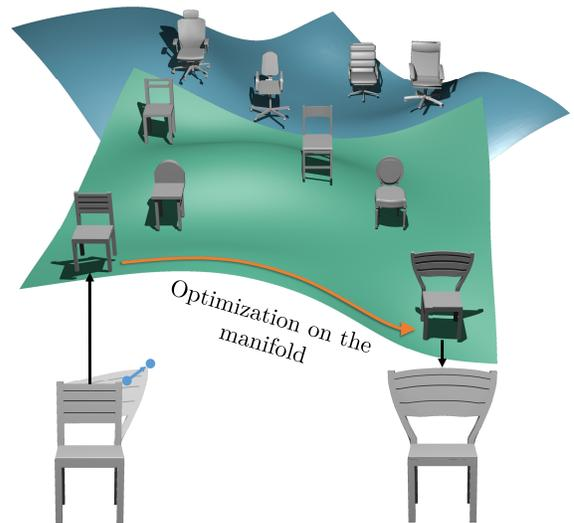
**Figure 1:** Illustration of a disconnected manifold of 3D chairs, where a chair is optimized on the connected component it lies on to fit a user deformation and generate the expected realistic design.
