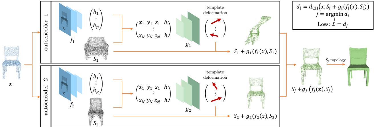
**Figure 2:** Illustration of the DiscoNet pipeline with  $k = 2$  autoencoders. The input  $x$  is reconstructed through both autoencoders, the best reconstruction being used as the output. Each decoder synthesizes the shape by warping its own pre-learned 3D template  $S_i$ .
