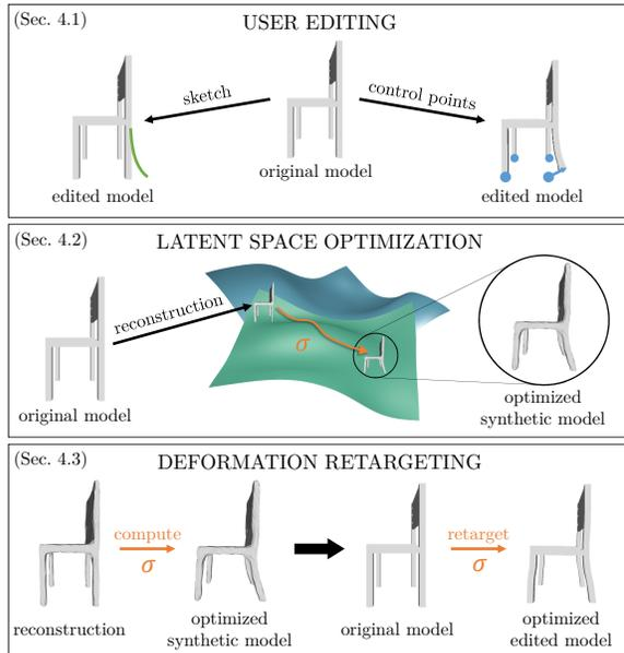
**Figure 7:** Illustration of our 3D editing pipeline: optimization on the learned shapes manifold to locally fit a user edit, and retargeting of the induced morphing onto the original model.
