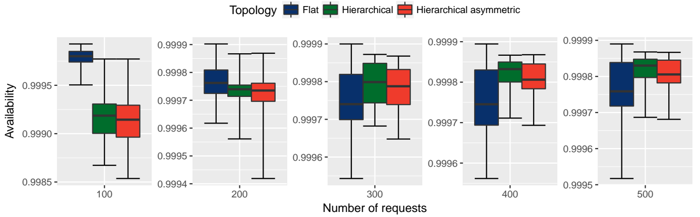
Figure 20: Availability of flat and hierarchical topologies when the number of requests increases.
