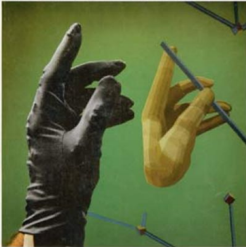
Wired Glove gives a computer user the sensation of handling objects on the screen: the image of the hand mimics the user's movements.
