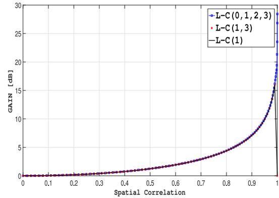
Fig. 4.  $G_B$  as a function of  $\alpha$ , circular Bernoulli impulsive interference.
