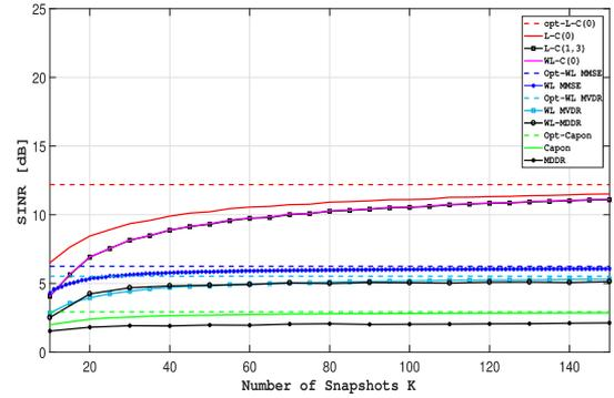
Fig. 7.  $\widehat{E}(\text{SINR}(K))$  as a function of  $K$  for a non-filtered QPSK SOI and a non-filtered BPSK interference.
