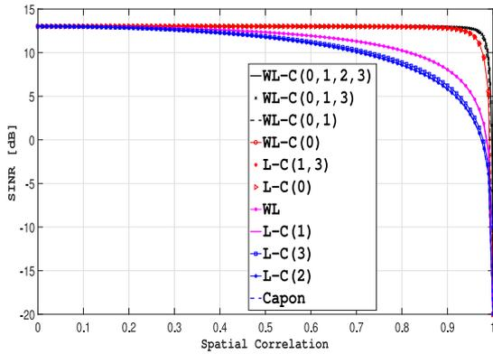
Fig. 2.  $SINR_B$  as a function of  $\alpha$ , non-filtered BPSK interference.
