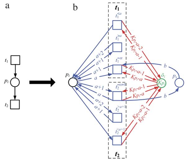
Fig. 6. (a) A subnet for  $p_i$  and (b) the supervisory structure for Eq. (16).
