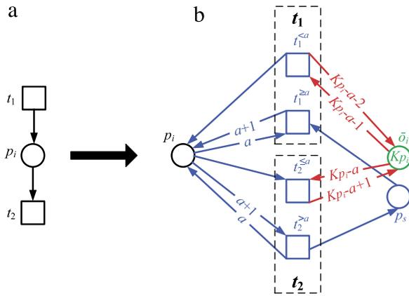
Fig. 5. (a) A subnet for  $p_i$  and (b) the supervisory structure for Eq. (15).
