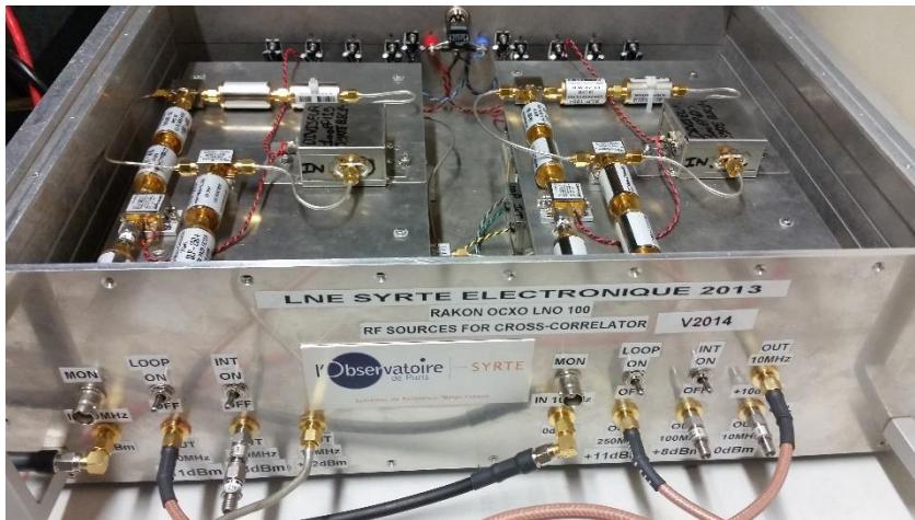
Photo of the frequency chain generating 2 ~statistically independant 250MHz clock signals (but f-locked at low Fourier frequencies)
