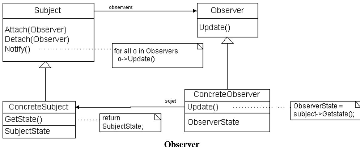
Initially, a concrete observer uses the abstract `Attach()` method to connect itself to one subject. The subject then keeps a reference to this new observer for further notification calls. The concrete subject will use the `Notify()` method when its internal state has changed. In `Notify()`, all the attached observers will be updated by invoking their respective `Update()` method.
