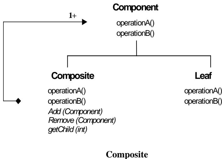
The standard Composite [GHJV95] [CS95] can apply operations uniformly on Composite and leaf nodes. Its implementation of operations allows recursive traversal of the tree transparently.
