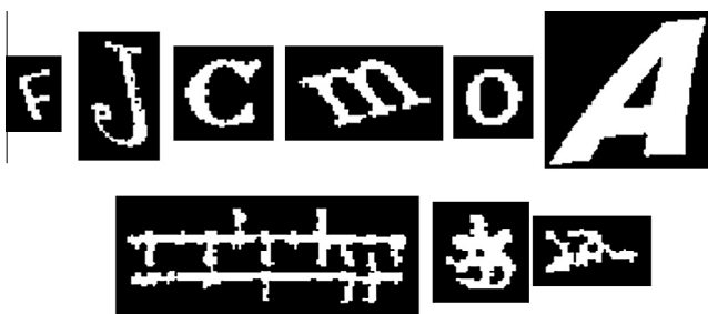
Fig. 13. Some of the positive samples (top) and negative samples (bottom) used to train the SVM shape classifiers for character/non-character discrimination. (Provided by Fabrizio [35].)
