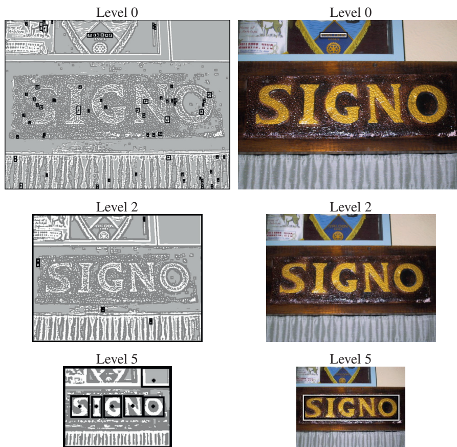
Fig. 12. Example of multi-scale segmentation and character filtering with reduction factor \mu = \sqrt{2} , illustrating suppression of spurious texture at the proper scale. Note that the characters of 'SIGNO' are over-segmented in levels 0 and 2 but correctly segmented and recognized (black boxes) in level 5.
