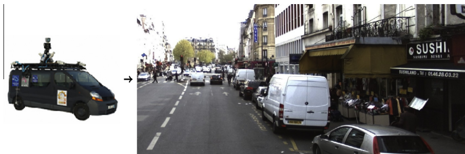
Fig. 1. The iTowns imaging vehicle and a captured image.
