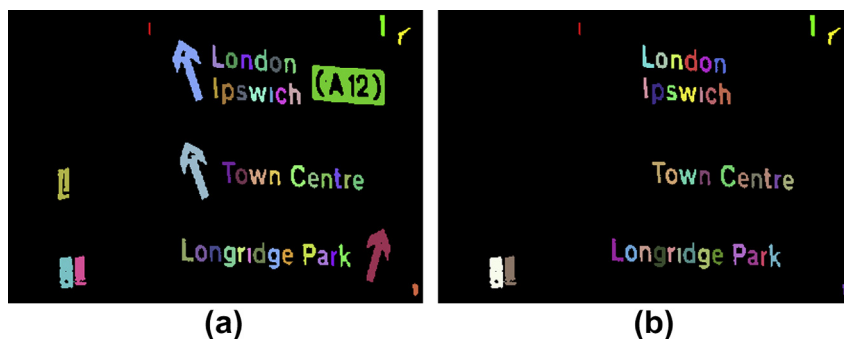
Fig. 6. (a) The foreground segments of Fig. 5(a) that satisfy the height and aspect ratio constraints with h_{\min} = 13 px, h_{\max} = 78 px, r_{\min} = 0.5 , and r_{\max} = 8.0 . (b) The subset of the segments in (a) that pass the character/non-character shape classifier.
