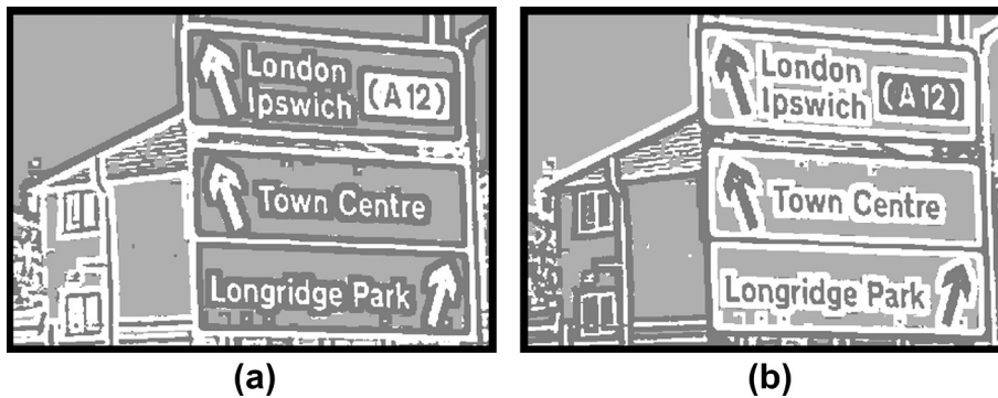
Fig. 5. (a) Toggle segmentation of the original image of Fig. 4 into background (dark gray), foreground (white) and indeterminate (light gray) pixels. (b) Toggle segmentation of the negative image.
