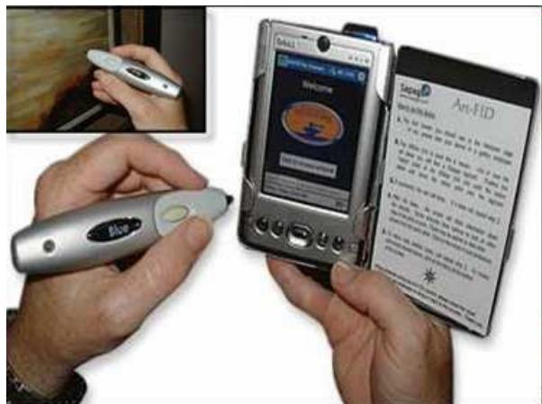
The gallery of art Granite State MetalWorks endowed its paintings With RFID chips containing data readable thanks to a bluetooth pe
